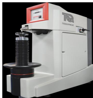
Rockwell Hardness Tester
