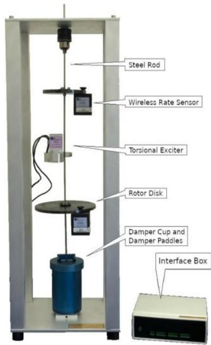
Torsional vibration system
