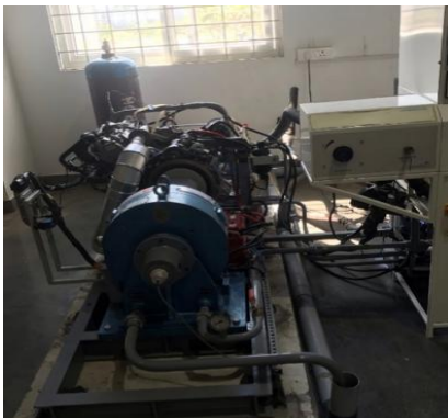
Two-cylinder CRDi Diesel engine setup
