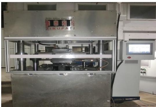
Abrasive flow finishing
