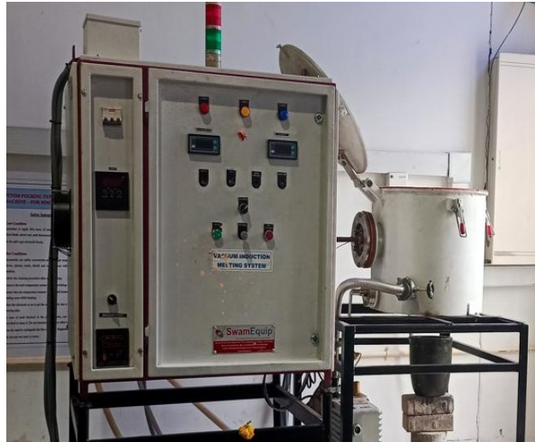
Vacuum Induction Furnace
