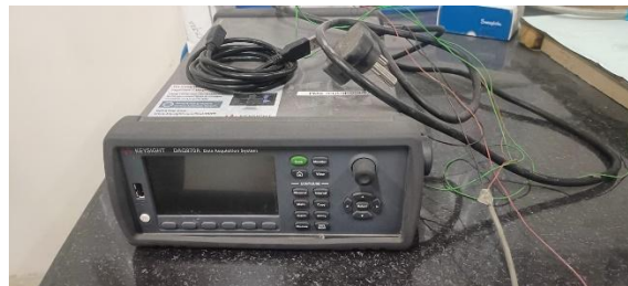
Data Acquisition system (DAQ)
