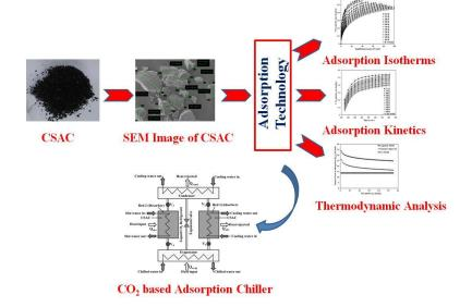
Development of adsorption chiller using coconut shell based activated carbon.
