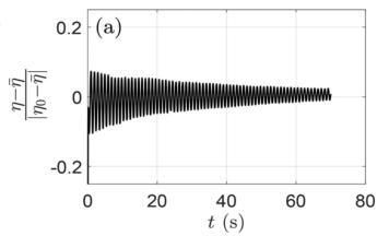
Wave damping in a rectangular tank:
