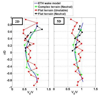
Comparison between the spatially-averaged spanwise profiles of wind speed measured using drone based wind measurement system under different atmospheric conditions and the predictions from the ETH wake model at two-diameter and five-diameter downstream of a wind turbine.
