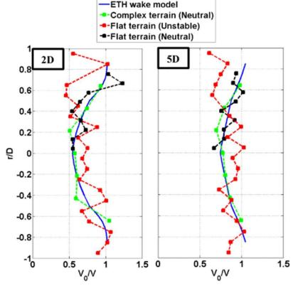
Comparison between the spatially-averaged spanwise profiles of wind speed measured using drone based wind measurement system under different atmospheric conditions and the predictions from the ETH wake model at two-diameter and five-diameter downstream of a wind turbine.
