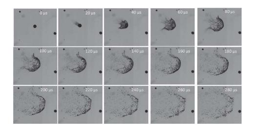
Image sequence showing micro-explosion of secondary droplets resulting from the explosion of suspended droplets. Micro-explosion of droplets start as strong puffing making droplet bag or sheet like structure before it breaks up into smaller droplets
